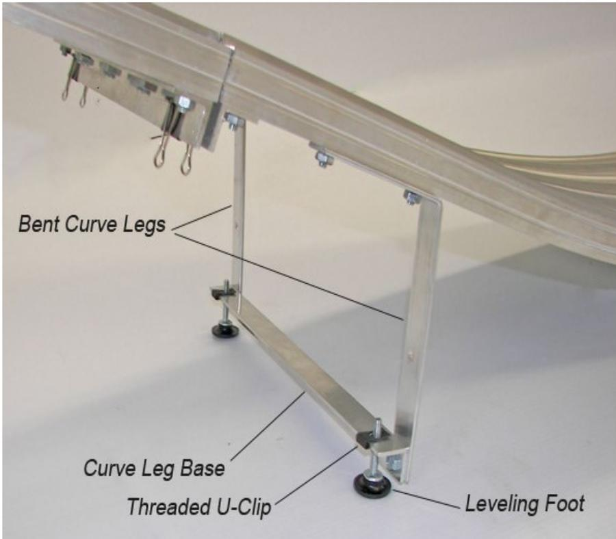
Install leveling mounts with leveling feet at the bottom end of the curve section as you did with the straight section. Attach these at the bottom end of your curve section as in the previous section.
