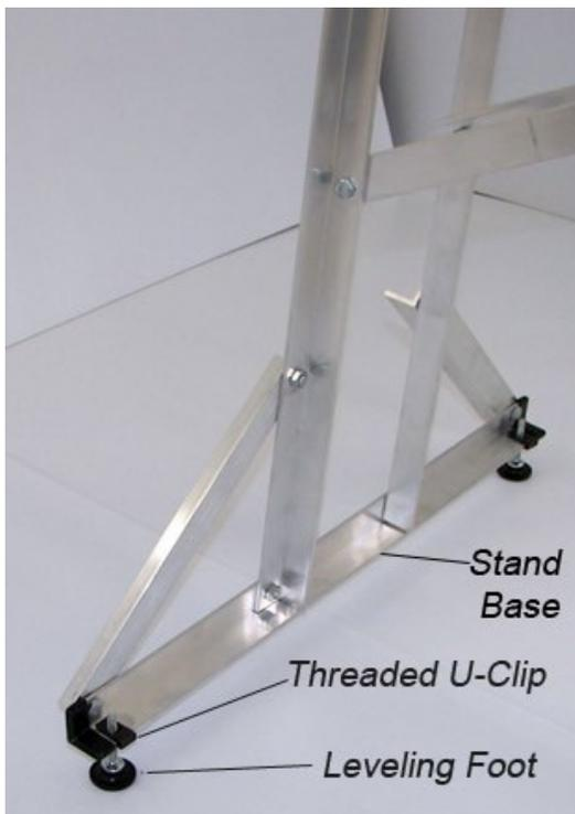
Snap two Threaded U-clips into the holes in the stand base. Thread a leveling foot into each U-clip.
