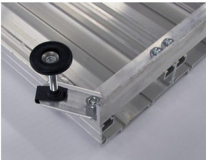
Starting with one section face down, remove only the nut at one end of a connector angle. Place the leveling mount over the bolt and replace the nut. Be sure to position the mount with the foot up as shown in the picture. The leveling mount can be positioned inboard or outboard on the track. Repeat for the other three corners of the track section.
